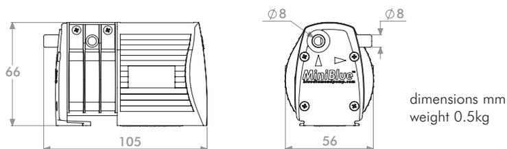
Patented rotary diaphragm pump
