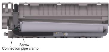
First remove the left side of evaporator from the groove of bottom shell and then remove the right side from the clasp on the bottom shell.
