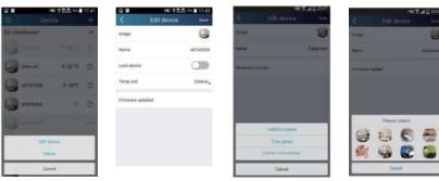
Step 2: Tap "Name" to change device name. Save it and the new device name will be shown. Enable button "Lock device" to lock the device so that other smart phones can't search the device. Tap "Temp unit" to change the temperature unit.
