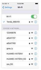
Step 2: In general, the hot spot signal of air conditioner is the last 8 bits of MAC address. Eg: Select "a0b41737" and enter the defaulted password "12345678" to connect it.
