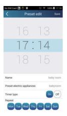
Step 2: Choose the time. Tap "Name". As shown in the picture, its name is "baby room". For timer type, select "On". Then select the repeating days. Save the setting of preset name.
