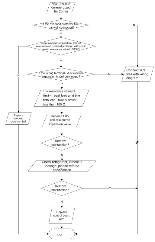
8.PFC (correction for power factor) malfunction (outdoor unit malfunction) (AP1 below is control board of outdoor unit)
